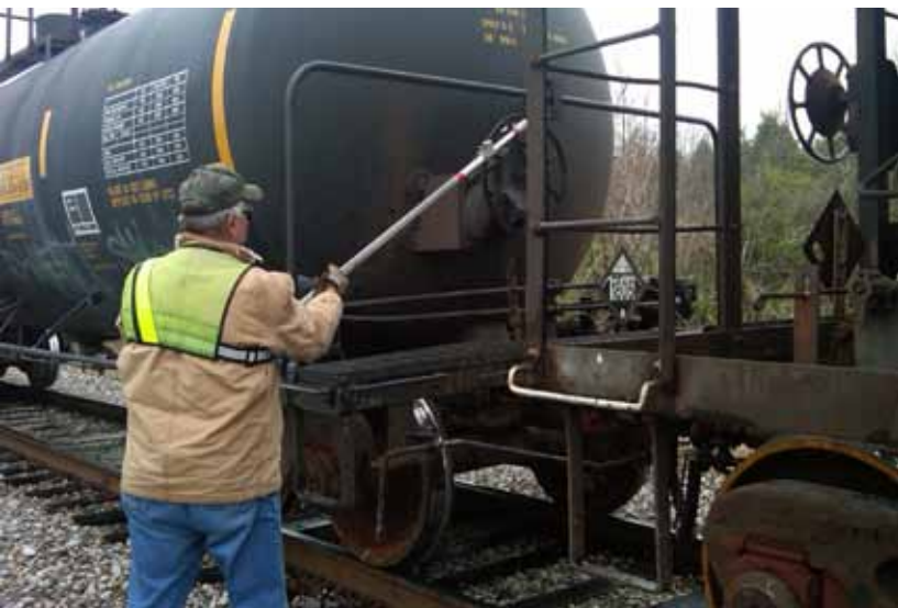
TSRR Conductor Rex Durham uses a new brake stick. The tool helps trainmen set the brakes without having to climb the car.
