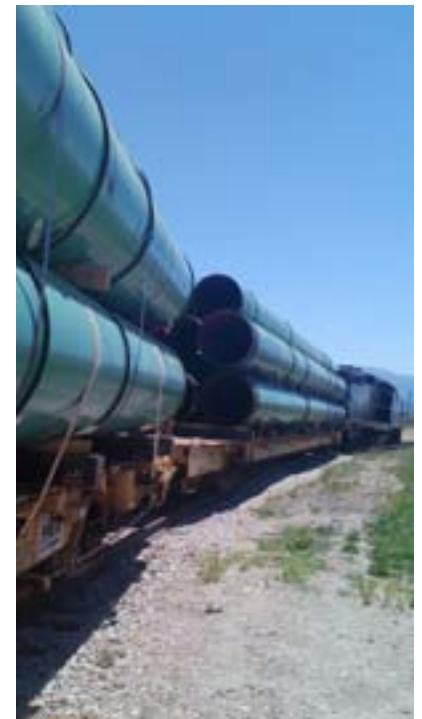
Each car carries approximately five 90-foot sections of steel pipeline.
