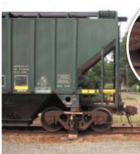
LEFT: From left, Harlan Dowdy, carman, and Marty Smith, lead carman, assist LNW at its Athens, La., transloading site. CENTER: A DQE jack lifts up an overloaded hopper car.
